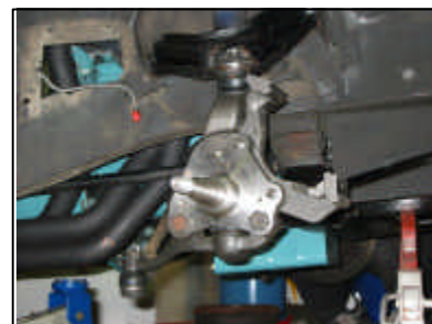
Front mounted caliper installation
